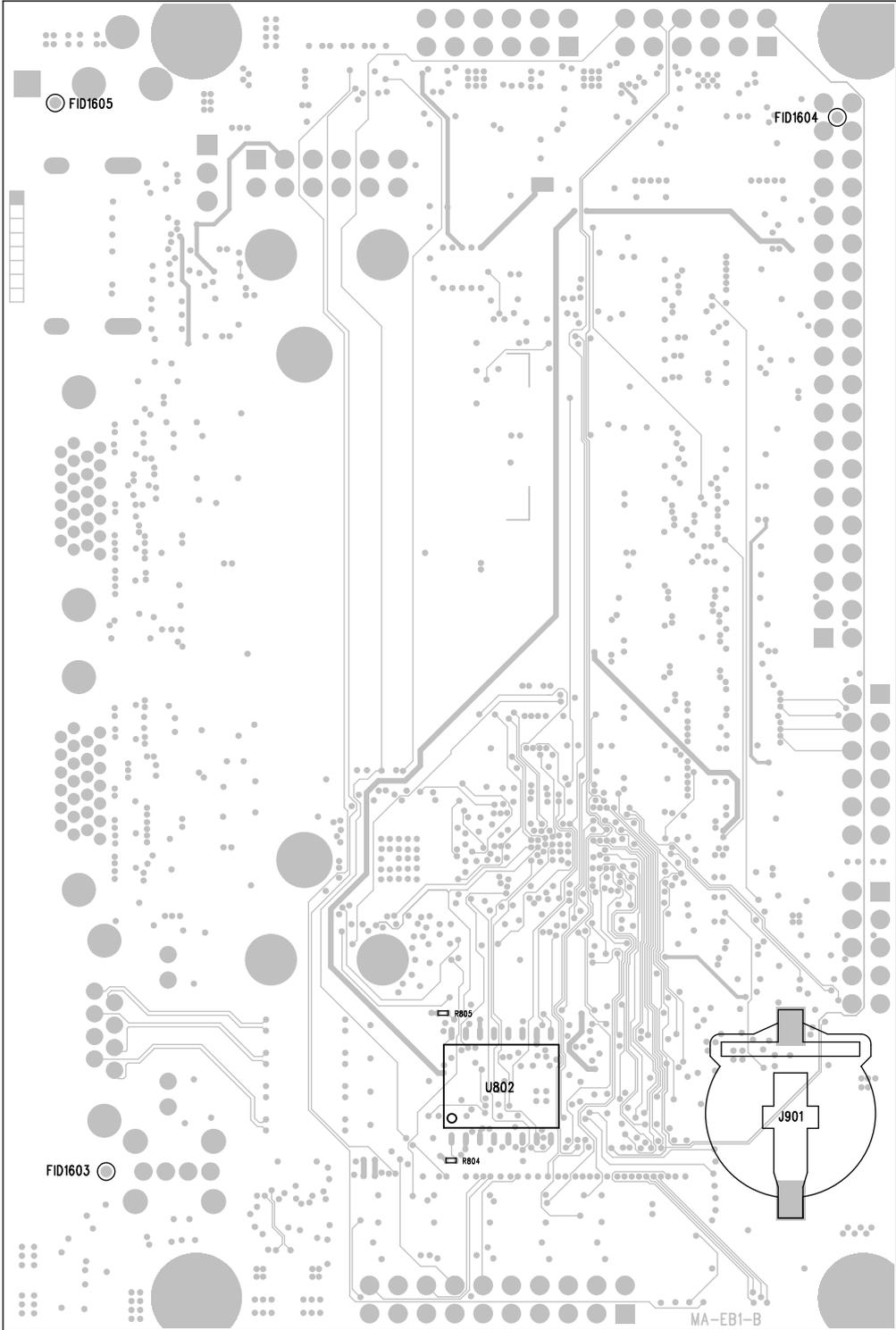
Figure 6: Board Bottom Assembly Drawing
