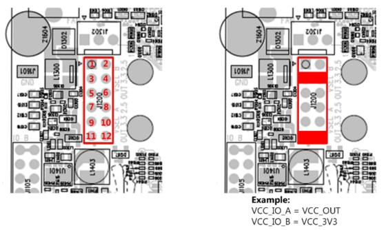
Figure 8: VCC\_IO Jumper Positions - Pin Numbering and Configuration Example
